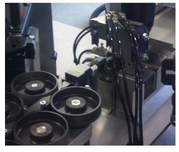
Feeder in the advanced position close to the cutting head, for the processing of very small section of cable. It can be powered that both roller belt
