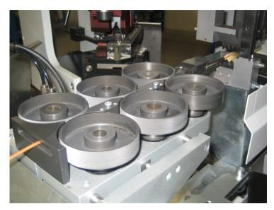
Feeder in the advanced position close to the cutting head, for the processing of very small section of cable.
