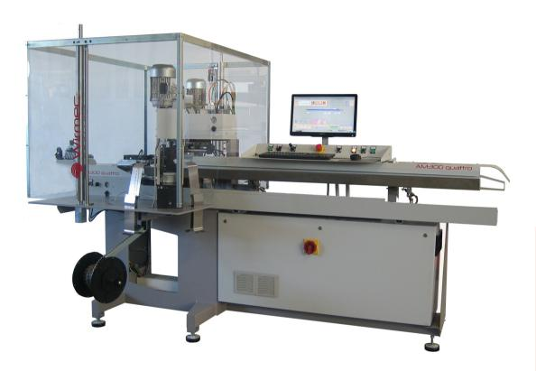
AM300 quattro is the ultimate expression of technology combined with Italian design. It is proposed as automatic cutting and stripping and crimping machine that can be equipped with up to five stations. It's projected for processing very small wire cross sections and very short wire lenght. Presents itself as machine as very simply and easy to use.
